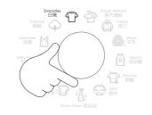
Select your desired wash cycle by turning the Control Dial. The wash cycle icons will illuminate as you turn the dial showing which cycle is selected, along with the default wash cycle settings.
