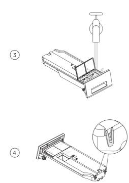
To clean the dispenser drawer, fill the compartments with warm water and shake lightly to clear residue. Drain all water from the compartments before re-fitting the dispenser drawer to the washer.
