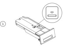
To remove the dispenser drawer from the washer, pull the dispenser drawer open, push down on the tab to the left of the **MANUAL DOSE** compartment and pull the dispenser drawer out from the washer.
