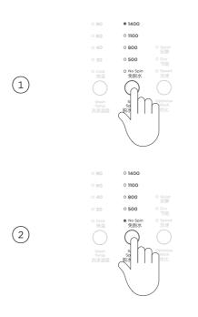
Press **SPIN SPEED** to select the required spin speed for your load.
