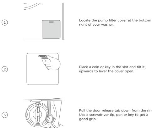
Place a coin or key in the slot and tilt it upwards to lever the cover open.
