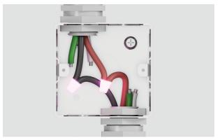
**3.** Connect the two black wires together with twist-on connectors and the two red wires together with twist-on connectors.
