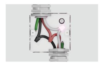
**4.** Seperate the green and white oven cable wires. Connect the white oven cable wire to the neutral (white) wire in junction box.
