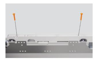
**1.** Unscrew the two Phillips screws to remove the top cover.
