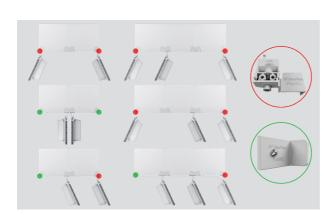
**3.** Fit either the depth gauges or spacers at the top and bottom of your product set based on your installation configuration.
