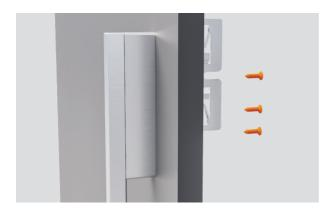
**7.** Fit the handle to the panels using four M5x25 hex screws. Ensure handle fixings do not interfere with side brackets.
