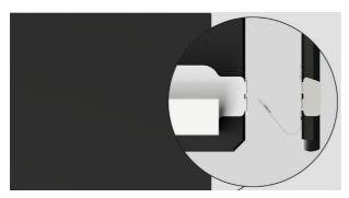
5. When replacing the second middle pane, ensure the metal bracket is still in place and correctly positioned at the bottom of the glass.
