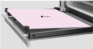
2. Pull pane towards the top of the door until clear of the brackets, then lift out.
