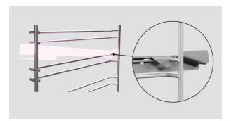
**4.** Ensure the rear tags are hooked over the side racks on both sides.
