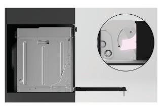
**3.** Push each locking lever down and lock into place. Ensure both hinges are fully locked before closing the door.
