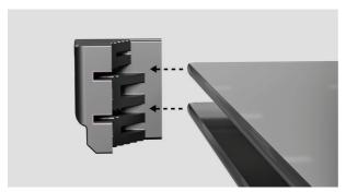
**2.** Ensure the rubber stoppers are attached to the glass and positioned correctly.
