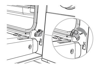
(1) Open the door completely, then open the levers on the left and right hinges to their full extent, as shown.
