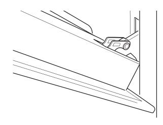
(2) Gently close the door until the left and right hinge levers are hooked to the door.
