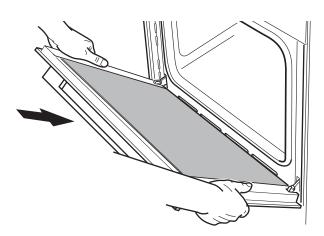
(1) Hold the door firmly and insert the hinge tongues into the slots on either side.
