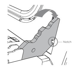
② Ensure that the notices on both sides drop into the places shown before opening the door to its full extent.
