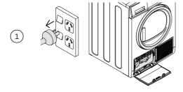
Switch off the power supply and remove the power plug.
