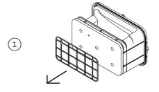
Remove the bracket securing the foam to condenser filter.
