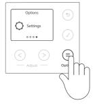
Press OPTIONS  $\equiv$ , scroll to SETTINGS using the ADJUST < > buttons, press  $\checkmark$  to confirm.
