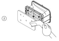
Remove the foam and vacuum lint build-up with a crevice nozzle.
