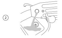
Pour the water down the sink or into a bucket, and then put the tank back in place.
