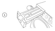
Remove the water tank by holding onto the handle and pulling outwards gently. Ensure the tank is kept level when removed to prevent the water from spilling.
