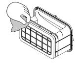
Use your hand, a cloth or a vacuum with a crevice nozzle to remove any lint build-up from the mesh surface of the filter.
