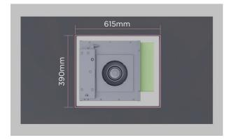
2. Create a 615x390mm cutout in the base of the cavity for the external blower.
