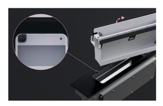
2. If required, lift the inner box out of the chassis. Remove both downdraft alignment guides and refit on the opposite side.
