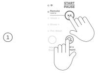
Press and hold ►II and ◯\\ ADD A GARMENT buttons for three seconds.
