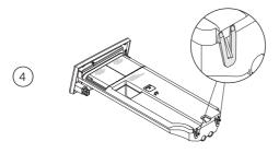
To disassemble the dispenser drawer further for cleaning, unhook the two clips at the rear of the dispenser to remove the cover.
