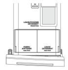
Add the washing machine cleaner directly into the MANUAL DOSE DETERGENT COMPARTMENT.
