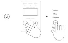
Press MORE +, LESS - and OPTIMISE WASH buttons together for three seconds, dEF will appear on the screen and the washer will beep.
