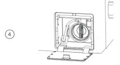
Refit the filter and turn clockwise to secure. The handles should be in the vertical position. Do not use excessive force to tighten.
