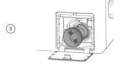
Turn the filter anti-clockwise to remove. Clean and rinse under a tap. Check and clear the cavity behind the filter. Remove any obstructions and check the impeller behind the filter moves freely.
