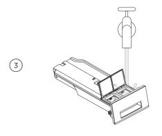
To clean the dispenser drawer, fill the compartments with warm water and shake lightly to clear residue.
