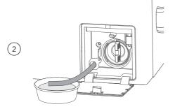
Unhook the outlet hose and pull it out (approximately 150mm). Remove the plug and allow any water (approximately 250ml) to drain into a shallow dish.
