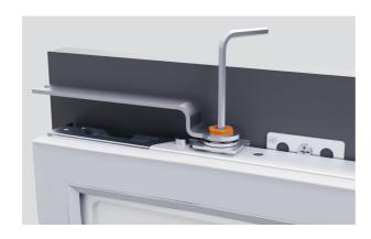
**8.** Tighten the M8 washers using the supplied spanner and hex key.
