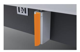
**3.** Using a box cutter, trim the supplied seal to length and clip onto the flow divider.
