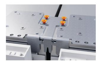
**3.** Secure the upper front bracket using four screws.
