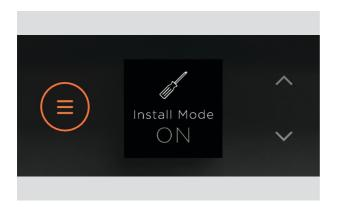
1. Press and hold  $\ \equiv \$  to exit install mode
