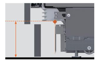
2. Measure the distance from the floor to the bottom of the grille to determine the position of the toe kick mounting plate.
