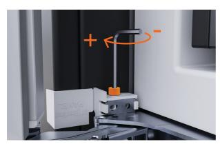
**6.** Expand the lower spacer to create an even gap between product and alcove.
