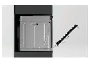
**3.** Holding the door on both sides, partially close the door and carefully pull the door away from the hinges.
