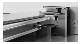
**3.** Slide the bottom of the glass into the lower brackets at the bottom of the door.
