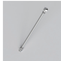
Hot water line with ferrule and compression nut - min 3/8" (9.5mm) copper tubing or flexible braided hose
