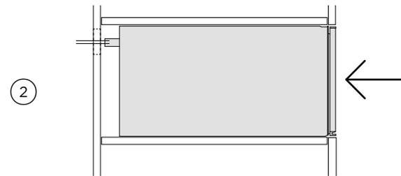
Push the warming drawer back into the cabinetry, and align the front panel with the cabinetry as desired.
