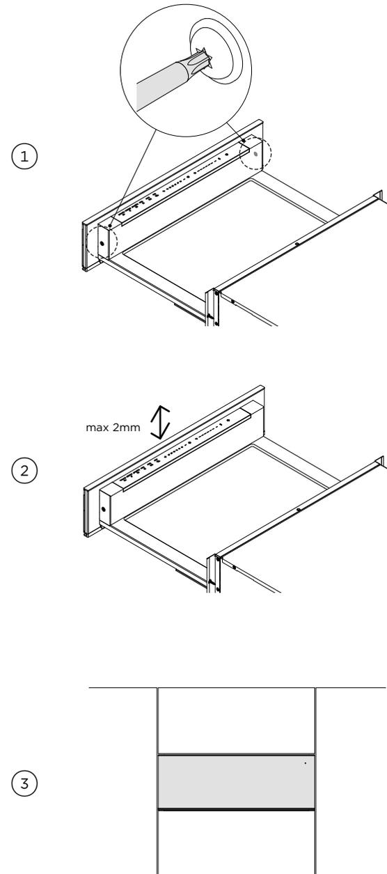
Open the drawer fully, and slightly loosen the screws.
