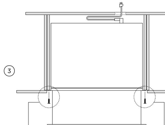
Open the drawer and secure the attachment flanges of the drawer to the side edges of cabinetry with 4x25 T20 star head countersunk screws.
