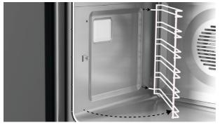
**3.** Pull the front of the rack clear of the screw and slide forward to remove.
