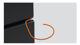
2. Carefully insert the door opener at the top right of the oven, between the centre louvre and the top of the door.
