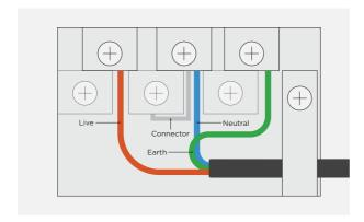
2. Based on your terminal block configuration, connect wires as shown. Connector and ports may not be present on all models.
