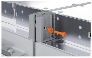
**3.** Clamp the upper brackets together by fitting the first the supplied M5 bolt and joiner sleeve. Tighten using a 8mm socket and Phillips screwdriver until the sleeve sits flush.
