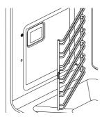
Slide the side rack forward until the rear tabs are clear of the mounting studs.
