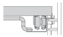
Ensure sliding shelves are positioned on top of the side rack wires instead of between them.
