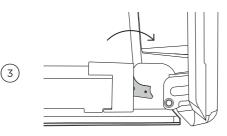
Ensure the levers are both fully locked before trying to shut the door.
