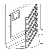
Slide the rear tabs of the side rack back onto the mounting studs, ensuring the rack is firmly pushed up against the side wall of the oven.
