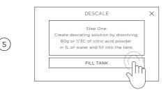
Fill tank with 4 cups (1L) of descaling solution<sup>\*</sup> and select **FILL TANK** to begin process.
