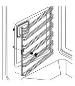
Unscrew and remove the fixing nut at the front of the side rack. Use a coin to loosen the nut if necessary.
