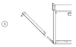
Holding the door on both sides, lift door back up to  $45^{\circ}$  and carefully pull the door out and away from the hinges.
