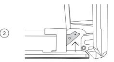
Push each locking lever up fully to release the door from the hinge.
