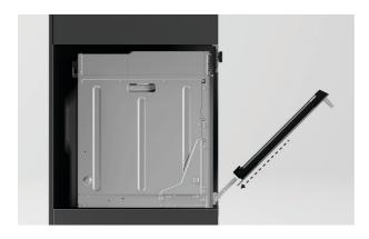
1. Holding the door on both sides, carefully lift door back onto the hinges.
