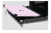
Pull the pane toward the top of the door until clear of the brackets, then lift out.
