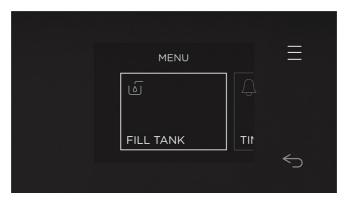
Press to open the water tank compartment.
