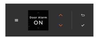
2. Press ✓ or ↑ to scroll to the desired feature and press ✓ to select.
