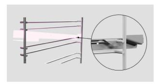
**2.** Ensure the rear tags are hooked over the side racks on both sides.
