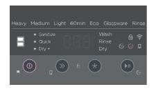
Press ① to select the drawer showing the alert, then press and hold ① for 2 seconds to clear the indicator.
