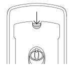
Press the latch down to open the dispenser. Check that the dispenser is empty and dry.
