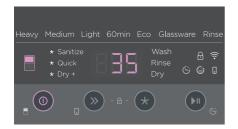
Press ① to switch between upper and lower drawers. The selected drawer will illuminate on the display.
