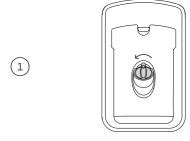
Turn the plug anticlockwise and remove.
