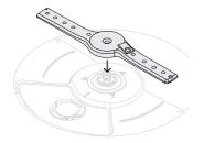
Place the spray arm to the impeller. Ensure the arm rotates freely when refitted.
