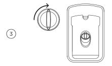
Refit the cap, turning clockwise until secure.
