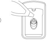
Pour rinse aid into the opening, taking care not to spill any into the drawer or on the aluminium handles.
