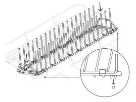
Align front and rear clips with the base rack and clip into place.
