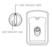
The salt reservoir is located on the inside of each drawer next to the detergent dispenser. It holds up to approximately 0.8lb (350g) of salt (actual capacity will vary depending on brand and grain size of salt used).
