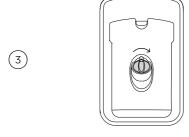
Refit the plug, turning clockwise until secure.
