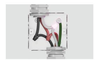
1. Seperate the factory-taped green and white oven cable wires. If junction box is grounded, connect the green wire to the metal junction box with a screw before connecting the white oven cable wire to the neutral (white) wire in juction box.
