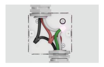
1. Connect the factory-taped gree and white oven wires to the neutral (white) wire in the junction box.
