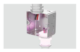
**2.** Connect the oven cable to the junction box through the U.L-listed conduit connector.
