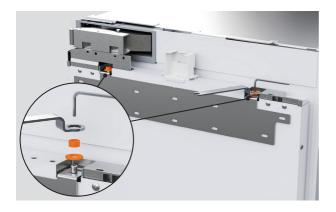
**1.** Remove the M8 nut and M8 washer from the M8 screw at the top of the door using the supplied hex key and spanner.
