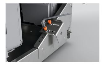
1. Loosen the adjustment bracket cap screws on both sides of the plinth using a hex key.
