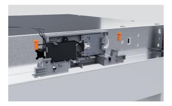
5. Reinstall the sensor housing using two #8x16 screws into the pre-drilled holes in the cabinet top panel.
