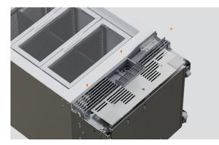
**4.** Secure with three #8x16 screws: one at the bottom left, one at the bottom right of the grille, and one behind the water filter hatch.
