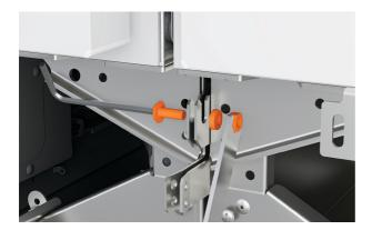
2. Secure the lower brackets together using the supplied M6 screw and Nut. Secure using a 4mm Allen key and 3/8" (10mm) spanner.
