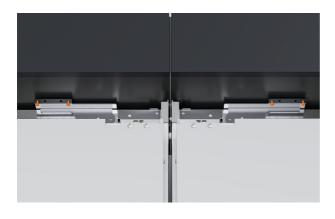
6. Fit the two upper brackets to the cabinetry using two 8Gx16 countersunk screws on each side.
