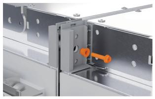
**3.** Clamp the upper brackets together by fitting the first supplied M5 bolt and joiner sleeve. Tighten using a 5/16" (8mm) socket and Phillips screwdriver until the sleeve sits flush.
