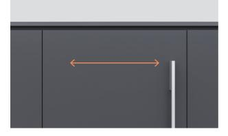
6. Push panel side-to-side to adjust horizontally. Ensure panels are flush with the front of the cabinet.
