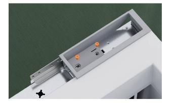
2. Install the new hinge pocket and alcove top bracket on the new hinge side using two M6x16 countersunk screws.
