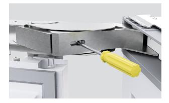
**1.** Release the hinge spring by turning the T20 screw in the hinge to the '0' position.
