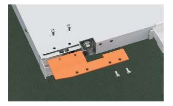
**1.** Unscrew the four M5x10 screws to remove the upper adapter bracket from the top of the door.
