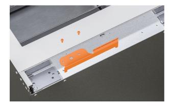
**5.** For the non-hinge side, remove the alcove bracket by unscrewing the M6x16 countersunk screws.
