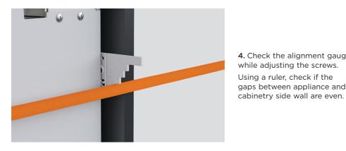
4. Check the alignment gauges while adjusting the screws. Using a ruler, check if the gaps between appliance and
