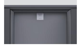
**2.** Measure the height from the floor to the front overhang and mark on the rear wall.
