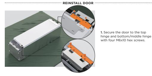
**1.** Secure the door to the top hinge and bottom/middle hinge with four M6x10 hex screws.
