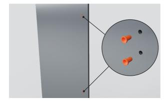
**2.** Remove the four plugs from the door panel.
