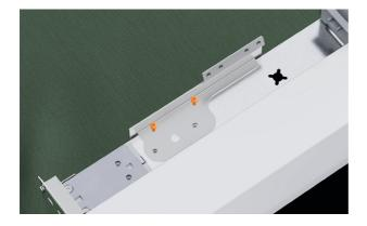
**5.** For the non-hinge side, fit a new alcove bracket using M6x16 countersunk screws.
