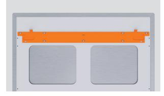
**5.** Secure the top hanging bracket to the screw holes of the door panel with M5 x 12 PH Screws.
