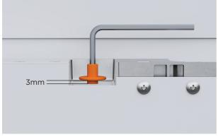
**3.** Loosen the M8 screws by 3mm.
