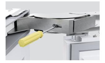
**2.** Activate the hinge spring by turning the T20 screws to the I position.
