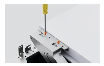
2. Detach the door from the appliance by unscrewing the door hinge M6x10 hex screws (4x) at the top hinge and bottom/middle hinge.
