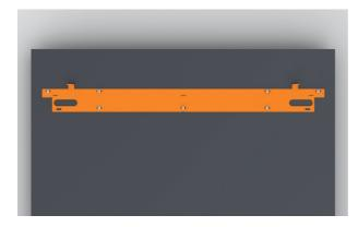
**2.** Align the door panel bracket to the panel. Secure using the supplied M5x12 screws.
