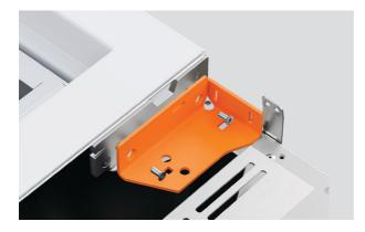
1. Fit a new lower hinge bracket on the new hinge side using two M6x16 screws
