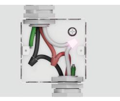
1. Seperate the green and white oven cable wires. Connect the white oven cable wire to the neutral (white) wire in junction box.
