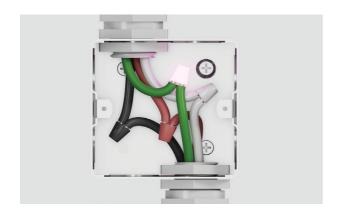
2. Connect the green grounding oven cable wire to the (green) grounding wire in the junction box. Do not connect the green grounding wire to the neutral (white) wire in junction box.
