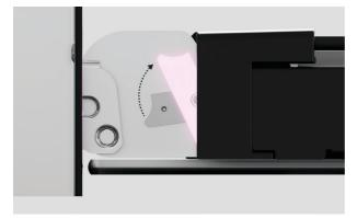
**3.** Locate the hinge locks on either side of the door. Push the locks upwards to release.
