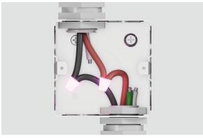
**3.** Connect the two black wires together with twist-on connectors and the two red wires together with twist-on connectors.
