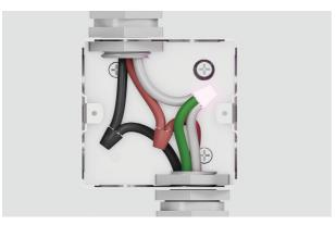
1. Connect the factory-taped gree and white oven wires to the neutral (white) wire in the junction box.
