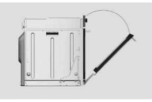
**4.** Holding the door on both sides, partially close the door and carefully pull the door away from the hinges.
