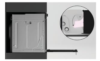
**2.** Open the door fully and push each locking lever down and lock into place.
