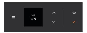
2. Press  $\checkmark$  or  $\land$  to scroll to ICE, then press  $\checkmark$  to turn the ice maker on or off.
