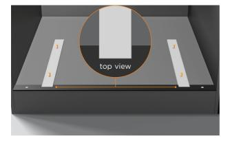
2. Slot the two side spacers into place. Ensure spacers are evenly spaced at the front and rear of the cavity.
