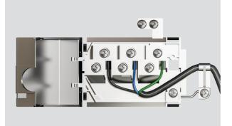
**2.** Connect to terminal block as shown. Ensure oven is correctly Earthed and cable clamp is tightened before closing the cover.
