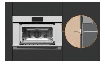
**2.** Secure oven to cavity using the 2 x #7x13 Phillips screws provided.
