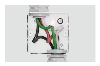
6. Connect the green grounding oven cable wire to the (green) grounding wire in the junction box. Do not connect the green grounding wire to the neutral (white) wire in junction box.
