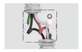
**5.** Seperate the green and white oven cable wires. Connect the white oven cable wire to the neutral (white) wire in junction box.
