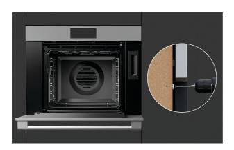
**3.** Secure oven to cavity using the 2 x #8x22 pan head screws provided.
