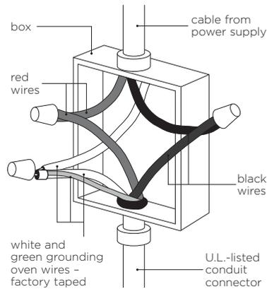
**If local codes permit connecting the cabinet-grounding conductor to the neutral (white) wire in the junction box:**
