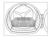
To remove the drying rack, tilt the top of the rack towards you this will detach the legs from the slots in the lint filter, gently remove from the drum. Check the lint and condenser filters are clean and replaced correctly before every load. Ensure the water tank is empty or drain hose secure before using your dryer.
