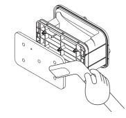
Remove the foam and vacuum lint build-up with a crevice nozzle.
