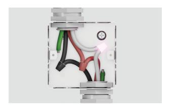
1. Seperate the green and white oven cable wires. Connect the white oven cable wire to the neutral (white) wire in junction box.
