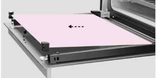
2. Pull pane towards the top of the door until clear of the brackets, then lift out. The rubber stoppers should remain attached to the glass.
