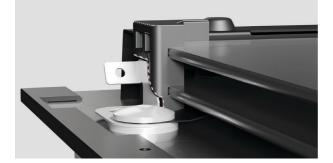
**4.** Lower the glass into place, with the rubber stoppers resting on the outer pane of glass.
