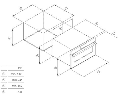
\*A 6mm panel spacer is required in the base of the cavity.
