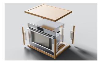
1. Cut all straps and remove the carton top cap. Lift the carton sleeve and remove any transit packaging. Set aside any accessories.
