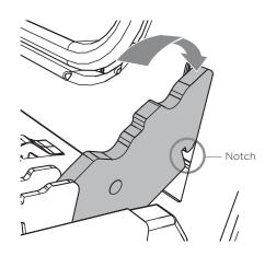
② Ensure that the notices on both sides drop into the places shown before opening the door to its full extent.
