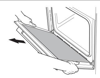
3 Hold the door firmly, as shown, and lift the door to remove.
