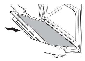
① Hold the door firmly and insert the hinge tongues into the slots on either side.
