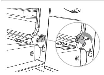
① Open the door completely, then open the levers on the left and right hinges to their full extent, as shown.
