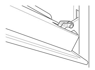
② Gently close the door until the left and right hinge levers are hooked to the door.
