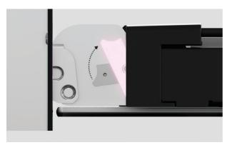
2. Locate the hinge locks on either side of the door.
