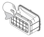
Use your hand, a cloth or a vacuum with a crevice nozzle to remove any lint build-up from the mesh surface of the filter.
