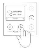
Select the desired cycle. Use the ADJUST < > buttons to adjust the time up or down. Press the ✓ button to confirm.
