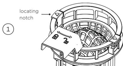
Align the filter cap with the notch on the
