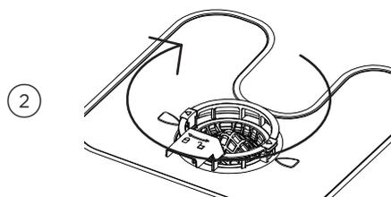
Place the drain filter back into the dishwasher
