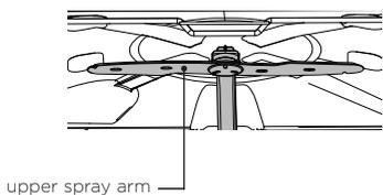
Do not remove the upper spray arm for cleaning.
