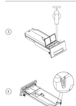
To clean the dispenser drawer, fill the compartments with warm water and shake lightly to clear residue. Drain all water from the compartments before re-fitting the dispenser drawer to the washer.
