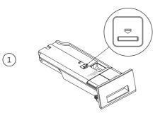
To remove the dispenser drawer from the washer, pull it open, push down on the tab to the left of the MANUAL DOSE compartment and pull it out from the washer.
