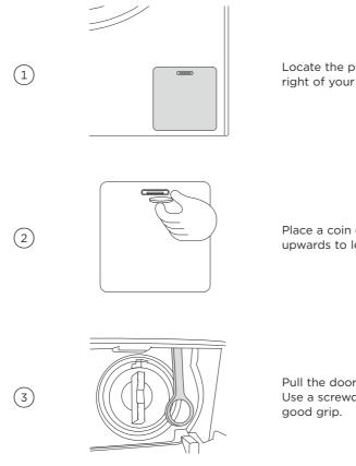
Locate the pump filter cover at the bottom right of your washer.
