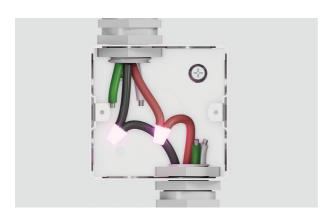
**3.** Connect the two black wires together with twist-on connectors and the two red wires togeher with twist-on connectors.
