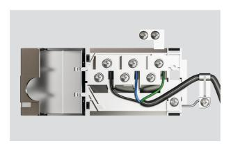
2. Connect to terminal block as shown. Ensure oven is correctly Earthed and cable clamp is tightened before closing the cover.
