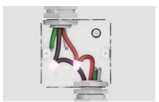
**3.** Connect the two black wires together with twist-on connectors and the two red wires togeher with twist-on connectors.
