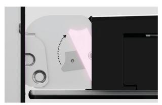
3. Locate the hinge locks on either side of the door. Push the locks upwards to release. Holding the door on both sides, partially close the door and carefully pull the door away from the hinges.
