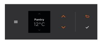
3. Press ✓ or ↑ to adjust the temperature, and press ✓ to confirm.
