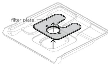
With the filter removed, carefully lift the filter plate up and out.
