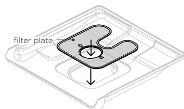
Slot the filter plate under the locating clips at the rear of the drain and push firmly back into place.
