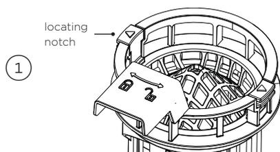
Align the filter cap with the notch on the filter base. Click together to secure.
