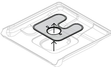
Remove the drain filter and the filter plate. Use a sponge to remove any remaining water from underneath before replacing.
