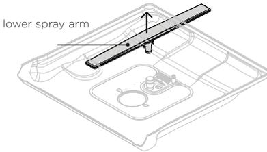
To remove the lower spray arm, lift it from the base of the dishwasher.
