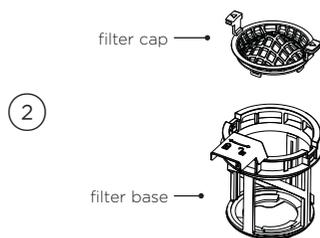
Separate the filter cap from the base by pressing the release buttons and lifting.
