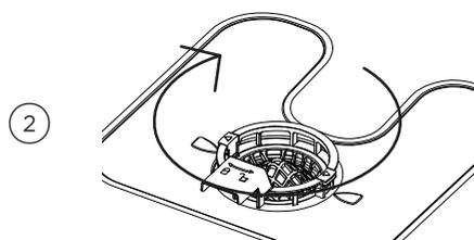
Place the drain filter back into the dishwasher base. Rotate clockwise to click into place.
