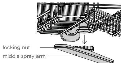
To remove the middle spray arm, turn the locking nut clockwise to release.
