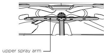
Do not remove the upper spray arm for cleaning.
