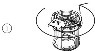
Twist the filter anti-clockwise to release. Lift to remove.
