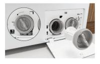
Turn the filters anti-clockwise to remove. Clean and rinse each filter. Check and clear the cavity behind each filter. Check the impeller behind each filter moves freely and remove any obstructions.
