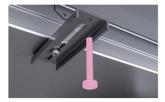
**2.** Tighten all clamp screws to secure the cooktops to the cutout and joiner strips.
