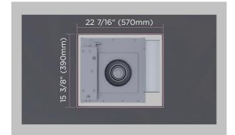
**2.** Create a 22  $7/16'' \times 15 3/8''$ (570 x 390mm) cutout in the base of the cavity for the external blower.
