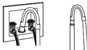
Installing the drain hose
