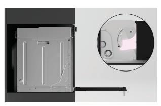
**3.** Push each locking lever down and lock into place. Ensure both hinges are fully locked before closing the door.
