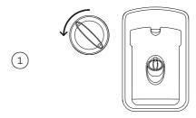
Turn the cap anticlockwise and remove.
