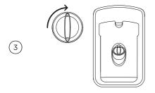
Refit the cap, turning clockwise until secure.
