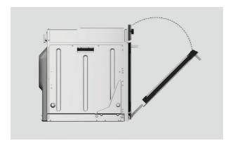
**4.** Holding the door on both sides, partially close the door and carefully pull the door away from the hinges.
