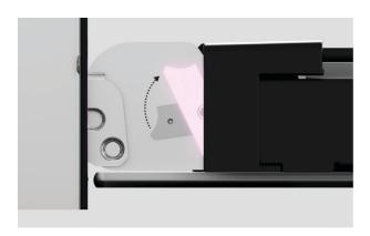
**3.** Locate the hinge locks on either side of the door. Push the locks upwards to release.
